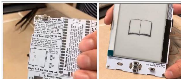
Figure 9: An 'alpha' prototype of TBBE by Joey Castillo from The Open Book project, with plans for custom PCBs through a multinational, cross-cultural collaboration for exhibition display.
