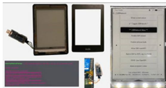
Figure 7: Subverting communication syntax technically, the paperwhite Kindle (top-centre) undergoes dual tapping through software (right side, bottom-left) and hardware (top-left, bottom-centre), with firmware reimaged to support both protocols.
