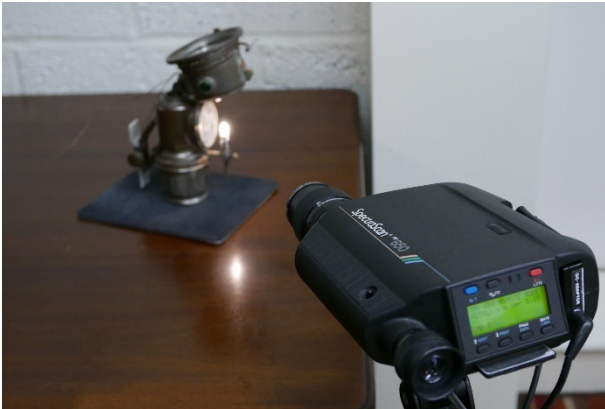
Figure 3: Measurement of flame spectrum with PR-650
