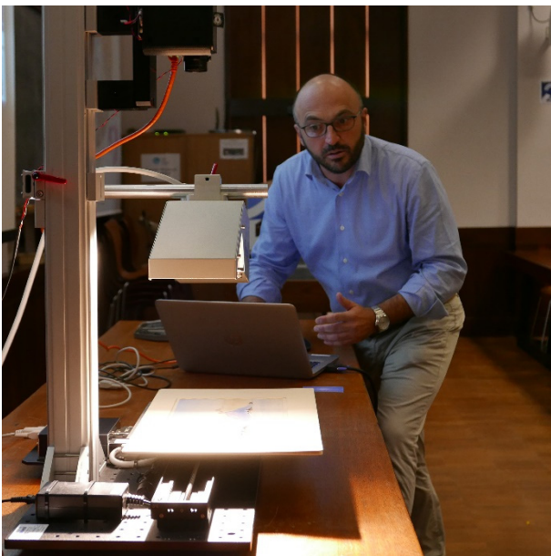
Figure 7: Dr Francesco Beccari with the Headwall hyperspectral scanner in operation at SPRI
