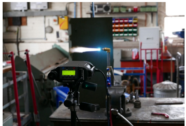
Figure 5: Measurement of an oxy-acetylene flame
